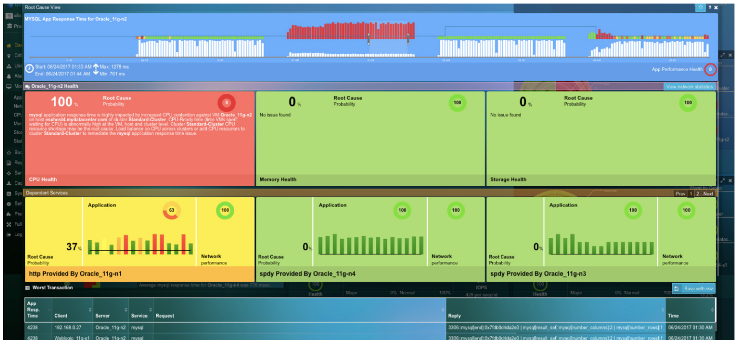
After clicking on an any application service on screen, Root Cause View automatically points out the root cause for the application performance degradation. In this case, the view shows the number of MySQL transactions and response times to and from a VM, including correlated performance metrics of the virtual / physical infrastructure and dependencies to other services. At the bottom are the application transactions (query/response) themselves, as well as their contents.
