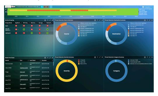
• Top of the Rack Switch visualization in the Network Traffic Flow Analysis view
